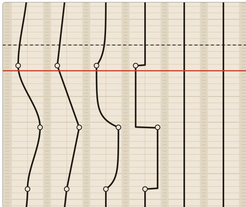
Figure 28. The same lanes as Glacial draws them, by its own code, the whole turn in view: S-curve, linear, exponential and step, in lanes 1 to 4; lanes 5 and 6 are blank, at 0 V. The drum stands an eighth of a turn past the seam, the dashed line above the playhead.
